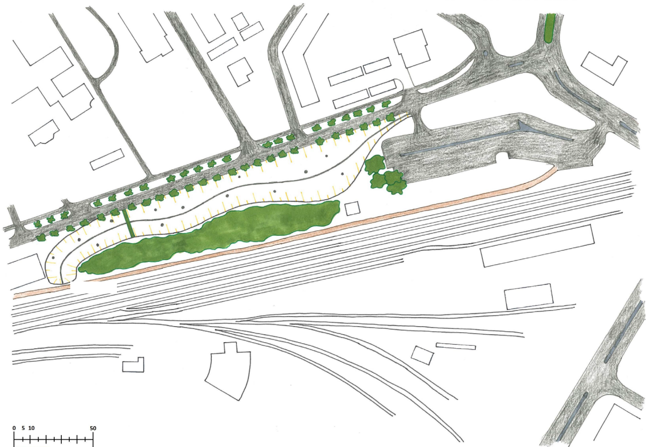
Drawing of the planned stormwater reservoir, designed as a park, with a dry stream bed.
