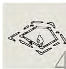
Set out the parts for each section onto the ground, assembling it like a jigsaw.
