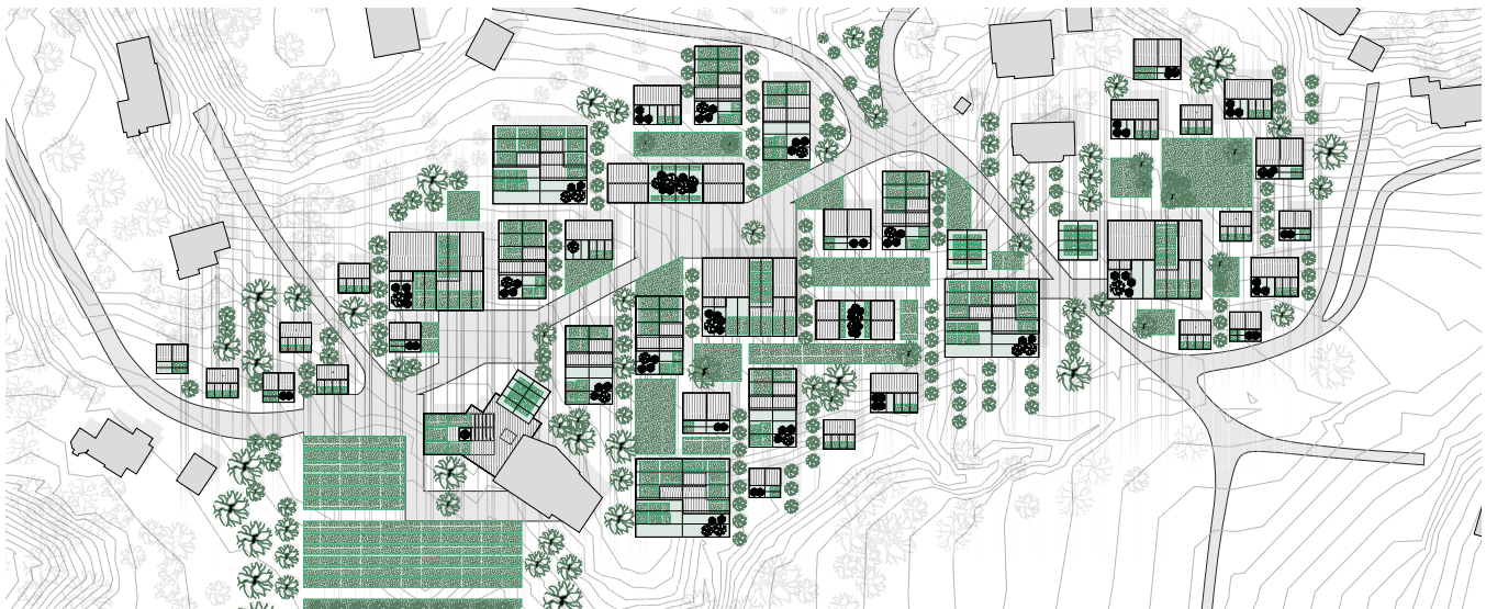
Figure 4. Greenhouses oriented South to benefit from optimal solar gain. Building thermodynamics reduce heating and cooling needs.
