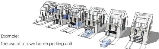
The robot parking flips up the garage door and sends the desired car to the front of the parking unit. The garage door functions as a rain shelter and the area to enter the car meets the dimensions for accessible parking. Therefore, all robot parking spaces can be considered accessible parking.
