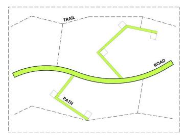
The main road will take the existing one. The old road will be adapted to the Project with new pedestrian an bicycle use. The second element, the path, will connect the productive blocks with the main road. Finally, a series of perimeter trails will enter the nearby forests and serve as a connection between the proposal and the nearby environment.
