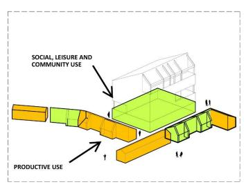
At the ground floor there are entrances to the auxiliary buildings. These buildings, apart from serving as support for the productive land, may also have leisure and commercial uses, creating relationships with the ground floor of the block. Greenhouses are located at the ends of these buildings and are dedicated to the productive use of micro-agriculture.
