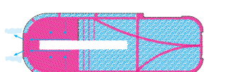
Water management Slight slopes collect water across the entire surface of public space and guide it towards vegetated weeds, dampening the effects of heavy precipitation
